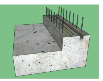
Using a natural bristle concrete brush coat the entire surface area of the cavity. Allow the application to dry for 1 to 2 hours.
